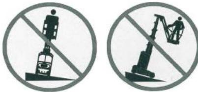
The tilt alarm cannot be used as a level indicator. Only when the machine is seriously tilted, the tilt alarm of the chassis and platform will sound.
