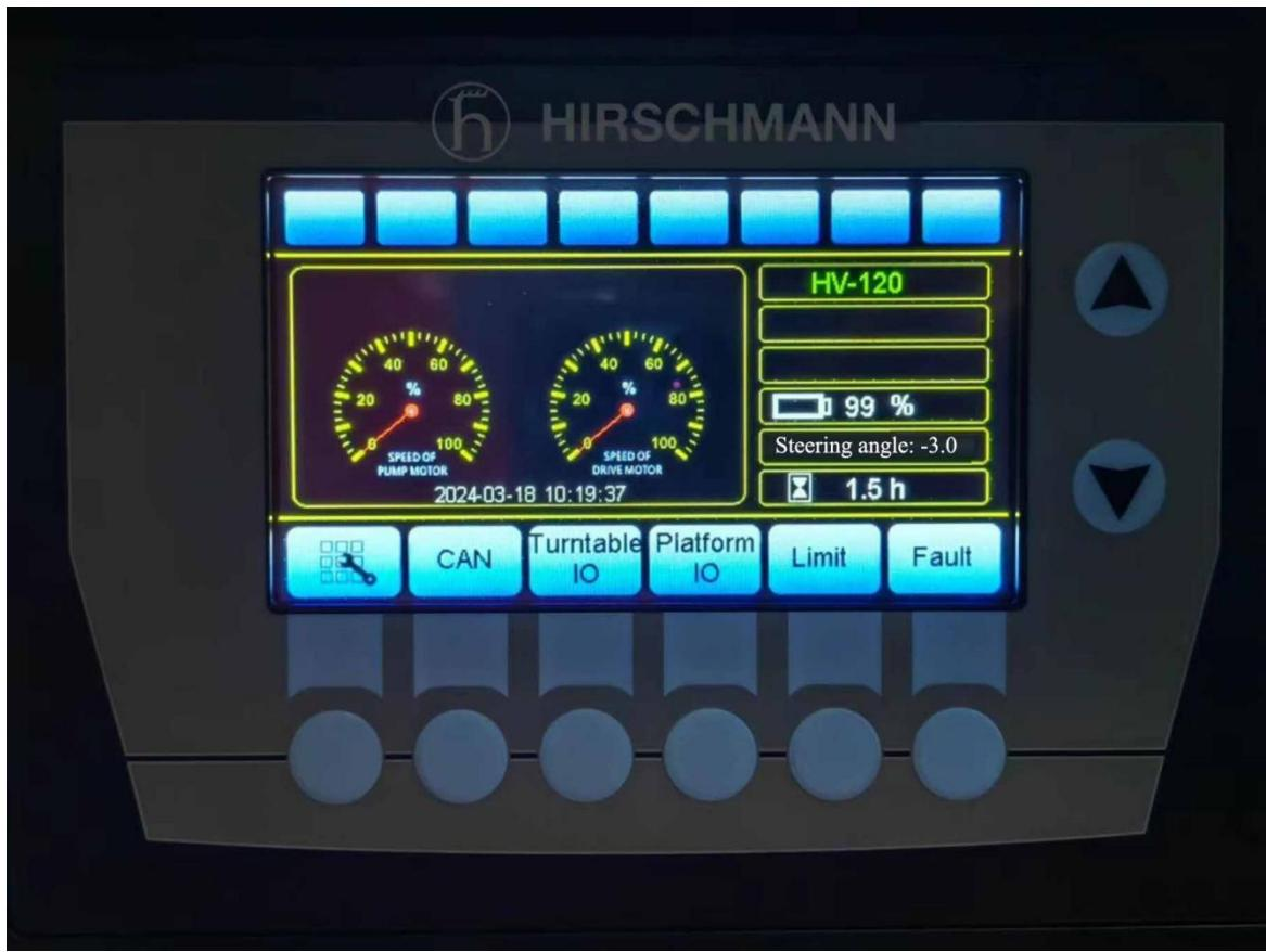
④ Result: No DTC shall be displayed on the display screen.
