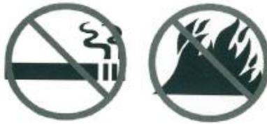
Keep sparks, flames and lighted cigarettes away from the battery. Batteries can give off explosive gases.
