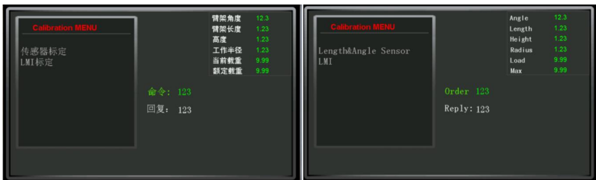
Figure 3.2.7.2-5 Schematic diagram of LMI calibration interface
