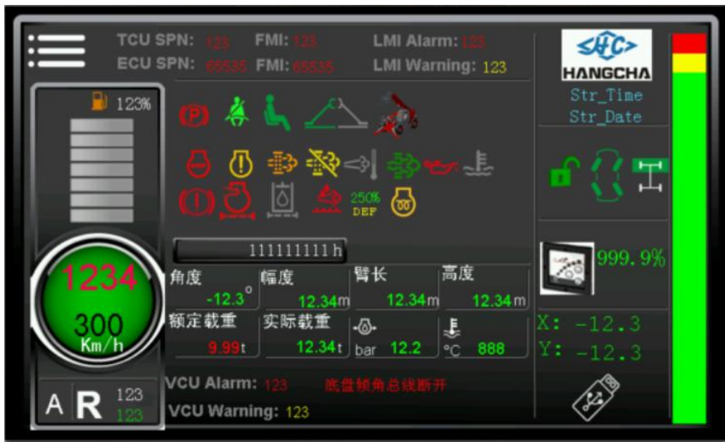
Figure 3.2.7.1-2 Schematic diagram of main interface buttons
