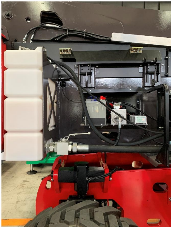
Hydraulic oil tank Location / 警示灯位置
